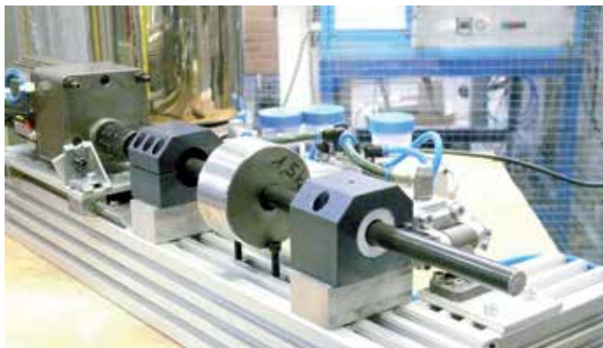
Two of our test benches for xiros® plastic ball bearings at igus® bearings laboratory
