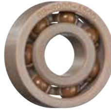
PEEK cage, PAI balls Temperature range -148°F to +302°F
